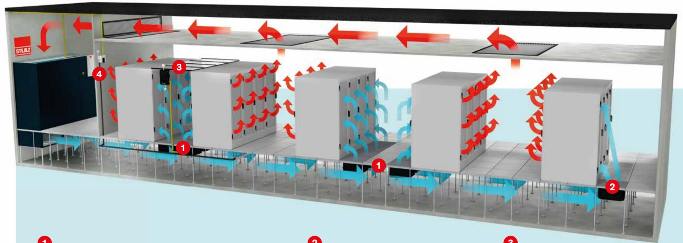
Airflow management solutions from STULZ are installed in the raised floors between server racks and air conditioning systems, and therefore utilize the air conduction of the air conditioning systems. Provided that the airflow in the raised floor is sufficient, the units supply your IT precisely according to cooling needs. Integrated sensors ensure that cold air requirements are automatically determined and the necessary airflow is provided. Fast, simple and reliable.
