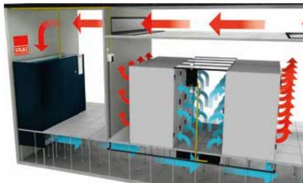
With needs-based airflow control, energy consumption for air conditioning in the cold aisle can be reduced. When several cold aisle enclosures are supplied from one raised floor, in particular, the varying heat loads of the individual aisles must be taken into consideration, to ensure constant server operating conditions. AirModulator 2 units are the ideal solution here.
